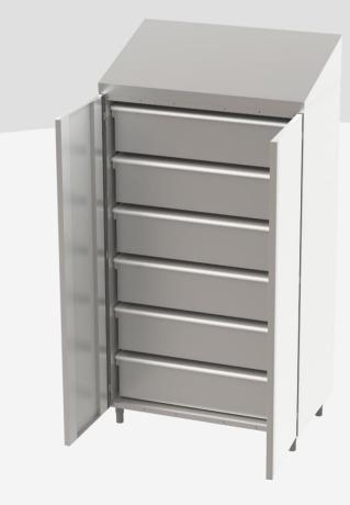
Made of AISI 304 Ni-Cr 18/10 stainless steel with Scotch Brite finish. Hinged doors mounted on hygienic hinges removable without the use of mechanical tools, with magnet closure. Complete with no. 6 box shelves H=300mm, complete with hinged lid in transparent polycarbonate. Space between each shelf 50mm. Prepared for wall mounting. On adjustable feet, the rear ones 80mm advances for rounded floor corner. Anti-dust inclined roof H=300mm.
