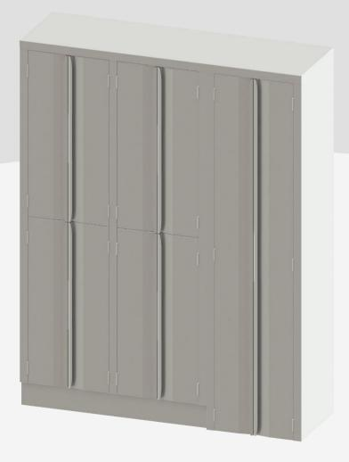
Made of AISI 304 Ni-Cr 18/10 stainless steel with Scotch Brite finish. On the left 4 compartments with 2 hinged doors and 1 height adjustable inner shelf each, dim. 600x535x1075Hmm. 1 compartment on the right with 2 hinged doors, dim. 2150x535x590Hmm. Hinged doors mounted on hygienic hinges removable without the use of mechanical tools, with magnet closure. On adjustable feet, the rear ones 80mm advanced for rounded floor corner. Plinth cover.
