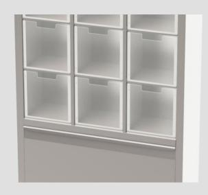
Made of AISI 304 Ni-Cr 18/10 stainless steel with Scotch Brite finish. Complete with 3 vertical rows of 4 compartments each, positioned on L-shaped runners welded to the structure, removable, with transparent polycarbonate front panels, internal dim. 347x330x350Hmm. H=500mm vasistas door at the bottom. On adjustable feet, the rear ones 80mm advanced for rounded floor corner. Prepared for wall mounting.
