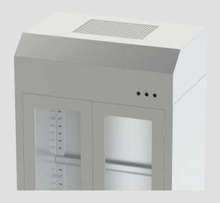
Made of AISI 304 stainless steel with Scotch Brite finish. Two hinged doors with stainless steel frame and 3 + 3 mm safety glass or 6 mm transparent polycarbonate, with 3 adjustable perforated shelves, made of AISI 316 stainless steel. On adjustable feet, the rear ones advanced 80 mm for rounded floor corner. Antidust inclined roof, with fan filter unit inside, 595x595x425Hmm
