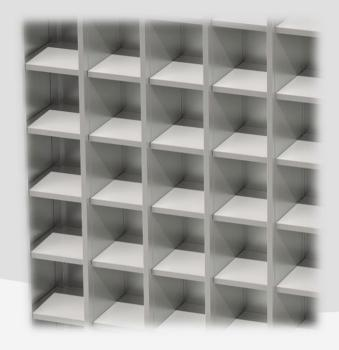
Made of AISI 304 Ni-Cr 18/10 stainless steel with Scotch Brite finish. Useful internal dimension of each compartment 200x250X200Hmm. Stainless steel telescopic feet, the rear ones 80mm advanced for rounded floor corner. Cover plinth.
