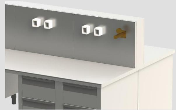
Made of AISI 304 Cr-Ni 18/10 stainless steel, Scotch Brite finish. Working top in AISI 304 sheet, 1.20mm thick, with inner plywood reinforcement and stainless steel lower cover. Rounded (R=10mm) front upper edge, as well as rounded (R=2mm) side and back edges. Central upstand H=500mm, rounded R10 on the lower edge, with screwed and removable back panel, holes for housing electrical sockets of your supply.
