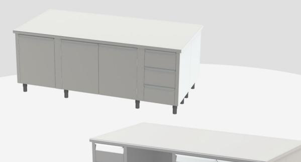
Made of AISI 304 Cr-Ni 18/10 stainless steel, Scotch Brite finish. Working top in AISI 304 sheet, 1.20mm thick, with inner plywood reinforcement and stainless steel lower cover. Rounded (R=10mm) front upper edge, as well as rounded (R=2mm) side edges. Left side from left to right:
