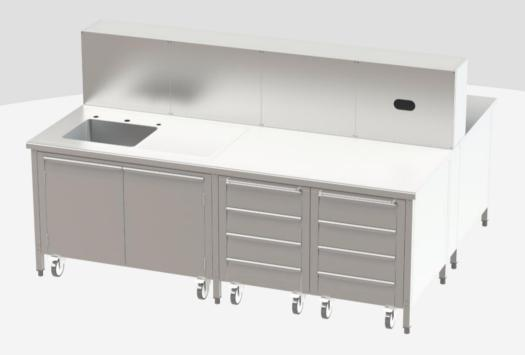
Made of AISI 304 Cr-Ni 18/10 stainless steel, Scotch Brite finish, with central structure for electrical sockets. Working top in AISI 304 sheet, 1.20mm thick, with inner plywood reinforcement and stainless steel lower cover. Rounded (R=10mm) front upper edge, as well as rounded (R=2mm) side edges. Central upstand H=500mm preapred for housing electrical sockets of your supply.
