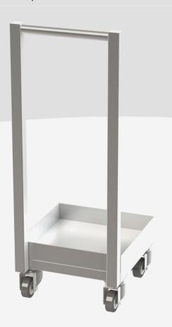
Made of AISI 304 stainless steel with Scotch Brite finish. Frame structure in 40x40mm tube, 2.00mm thick. H=30mm platform with perimeter edge H=52mm. Pull handle Ø25mm, H=704mm. Total height 793mm. On 4 swivel castors.
