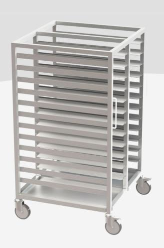
Made of AISI 304 Cr-Ni 18/10 stainless steel, Scotch Brite finish. Fully welded frame made of 30x30mm square tube, with upper and lower perimeter reinforcing frame. No. 12+12 pairs of welded rails complete with stops on both sides, useful dim. 356x730mm. No. 2 removable liquid collection tanks positioned on the bottom are included in the supply. Stainless steel round tube pull handle on the right side. On 4 swivel castors Ø125mm with stainless steel support, 2 with brakes.
