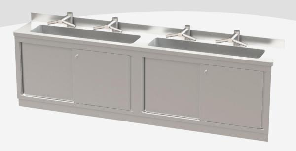
Made of AISI 304 Cr-Ni 18/10 stainless steel, Scotch Brite finish. Top with rounded R2 edges, and rounded R30mm front corners. No. 4 holes for Dyson mixer. Rear upstand H=100mm, welded and closed on the back. Sliding doors mounted on hygienic rails, easily removable without mechanical tools. Open back for hydraulic connections. PVC siphon, drain and stainless steel overflow included. Stainless steel supporting plinth advances on the back for rounded floor corner. Sink bowl dim. 1250x310x300Hmm.
