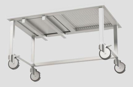
Frame structure in stainless steel AISI 304 fully welded 40x40mm tube, 1.00mm thick, rear legs 80mm advanced, suitable for rounded floor corner. Rear and side welded reinforcement rails. Working top in AISI 304 sheet, 1.50mm thick. Rounded (R=10mm) front edge, as well as rounded (R=2mm) side and back edges.
